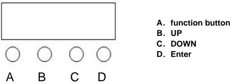
**Operation description:** Press "A" will cycle out seven different functional effect,LED Top row in represent the current function (Reference function table). LED Top row on behalf of the function in the address code, or speed and other parameters. Press B or C key can modify the parameter value. Press D to confirm.
