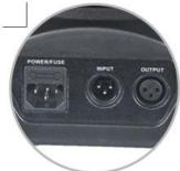
3-pin XLR signal connector input and output
