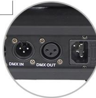
3-pin XLR signal connector input and output
