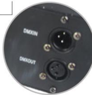
3-pin XLR signal connector IN/OUT
